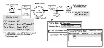
Figure 4: Voip Caller ID Case #4 - Remote FXS call on H.323 voip system
